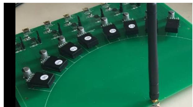
RF test fixture for testing 10 modules in parallel
